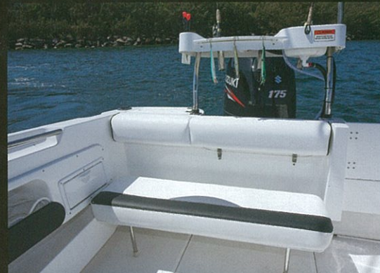
An aft lounge appears from the transom bulkhead on demand — and disappears completely when not needed.
